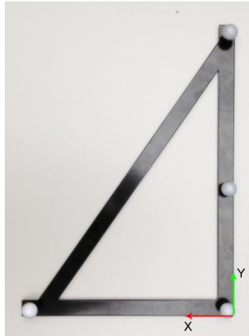
Figure 6.20. Device used for defining a reference coordinate system.
